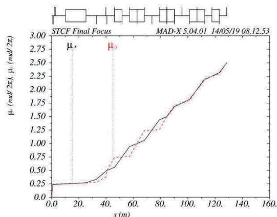
Figure 5: Phase advances of 1/2 final focus section.
