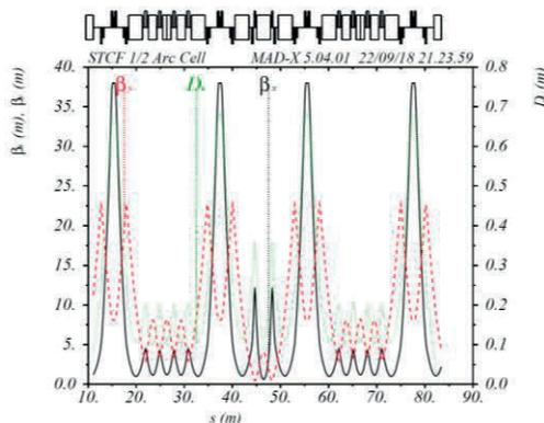
Figure 2: Sketchy design of the STCF 1/2 arc section.
