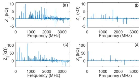
Figure 7: Wake impedance. (a): transverse wake impedance in X direction without ferrite load; (b): transverse wake impedance in X direction with ferrite load; (c): longitudinal wake impedance without ferrite load; (b): longitudinal wake impedance with ferrite load.
