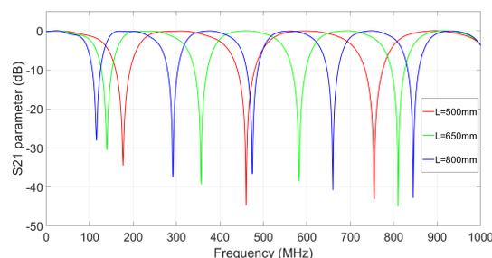
Figure 4: S21 parameter of the choke mode structure with different length of the radial line.
