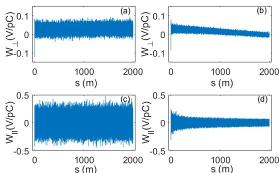
Figure 6: Wake potential. (a): transverse wake potential in X direction without ferrite load; (b): transverse wake potential in X direction with ferrite load; (c): longitudinal wake potential without ferrite load; (b): longitudinal wake potential with ferrite load.
