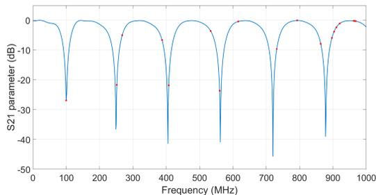
Figure 5: S21 parameter of the optimize choke mode structure.
