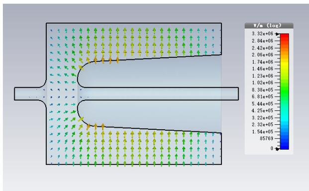
Figure 2: Electric field distribution for the first HOM mode.
