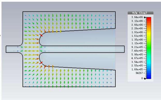
Figure 1: Electric field distribution for the fundamental mode.
