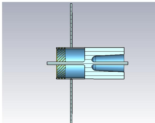
Figure 3: QWR cavity with choke mode structure.
