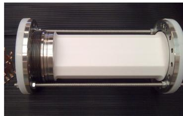
Figure 2: Ceramic vacuum chamber profile.
