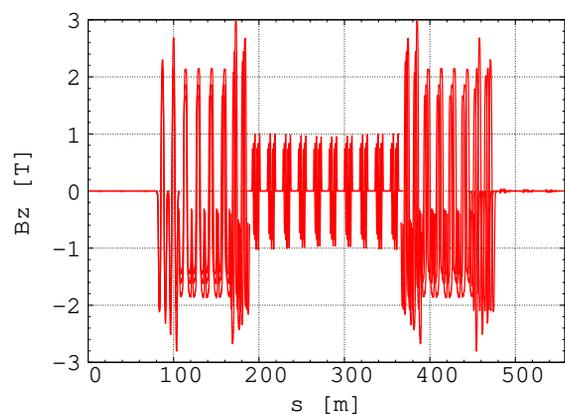
Figure 3: Vertical magnetic field on the median plane for the maximum circulating muon momentum in the ring (6.1 GeV/c). The plot is centered on the straight FFA part.
