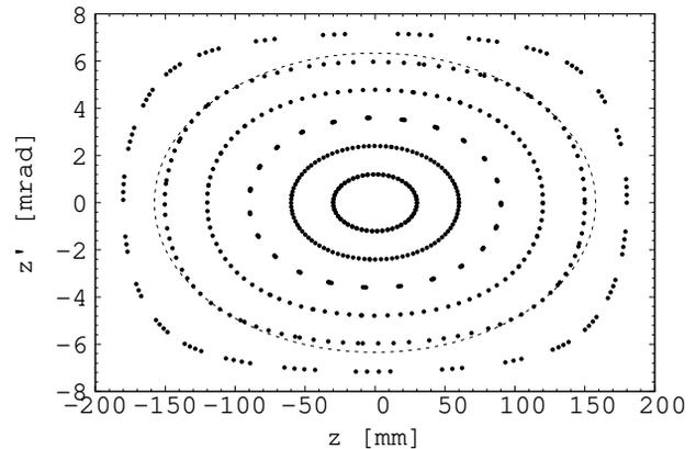
Figure 6: Stable motion in the vertical Poincare map for maximum initial amplitude over 100 turns for  $p_0$ . The ellipse shows a 1 mm.rad unnormalized emittance.
