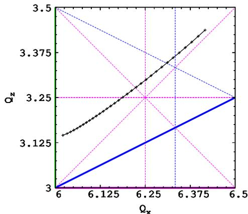
Figure 4: Tune diagram for momenta  $\pm 15\%$  around 5.3 GeV/c. Integer (red), half-integer (green), third integer (blue) and fourth integer (purple) normal resonances are plotted.
