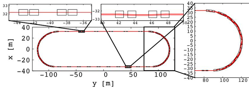
Figure 1: Top view of the racetrack hybrid lattice (bottom left scheme). The top left scheme shows a zoom on the production straight section, the top middle scheme the FFA straight part, and the right scheme a zoom on the arc section. Matched, minimum and maximum momenta muon closed orbits are shown in red. Effective field boundaries with collimators are shown in black.
