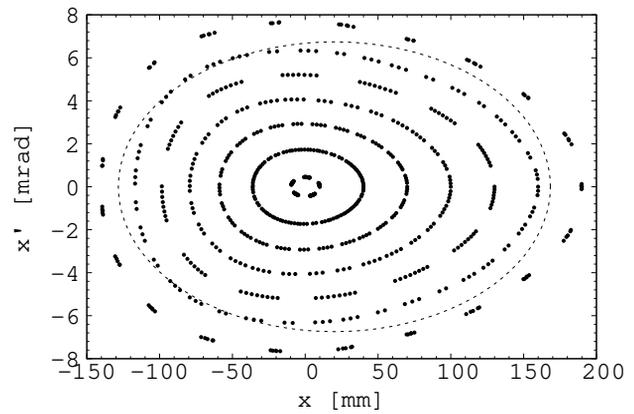
Figure 5: Stable motion in the horizontal Poincare map for maximum initial amplitude over 100 turns for  $p_0$ . The ellipse shows a 1 mm.rad unnormalized emittance.
