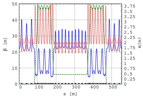
Figure 2: Horizontal (plain blue), vertical (dotted red) periodic betatron functions (left scale) and dispersion (mixed green line, right scale) in the ring for matching momentum. The plot is centered on the straight FFA part.
