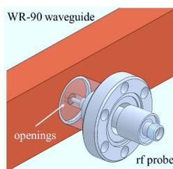
Figure 7: Design of the rf pickup. The pipe near the openings is set to be transparent to present the details.
