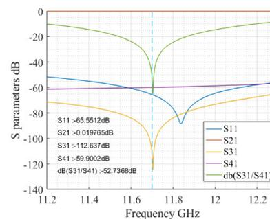
Figure 9: S-parameters of the directional coupler.
