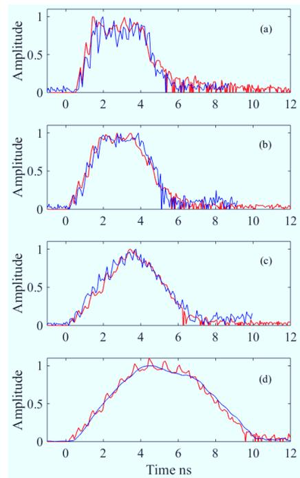
Figure 4: Comparison of the forward rf signal envelope between measurement (blue) and simulation (red) when driven by single bunch (a), 2-bunch train (b), 4-bunch train (c), and 8-bunch train (d).
