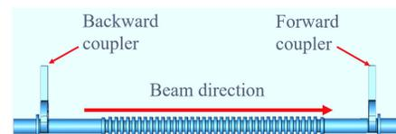
Figure 1: Layout of the X-band metallic power extractor.
