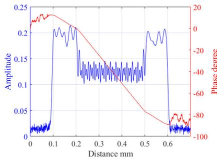
Figure 2: On-axis field distribution of the X-band metallic power extractor at 11.72 GHz. The phase velocity can be fitted from the slope of the phase distribution.
