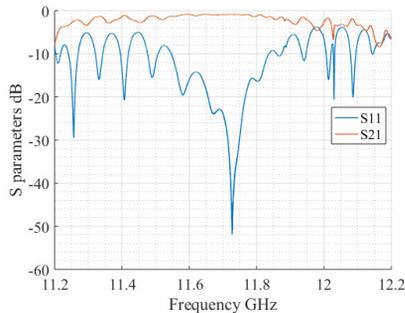
Figure 3: S-parameters of the X-band metallic power extractor. Port 1 and Port 2 are defined at the waveguide port on the backward and the forward coupler, respectively.
