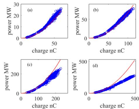
Figure 5: The measured forward rf power (blue dot) and the simulated value (red line) as a function of total transmitted charge when driven by single bunch (a), 2-bunch train (b), 4-bunch train (c), and 8-bunch train (d).
