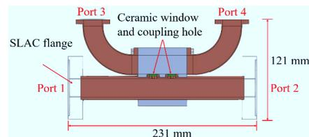
Figure 8: Layout of the directional coupler. Port 4 is used to measure the forward rf power going through Port 1 to Port 2. Port 3 is used to measure the reflected rf power coming from Port 2 to Port 1.
