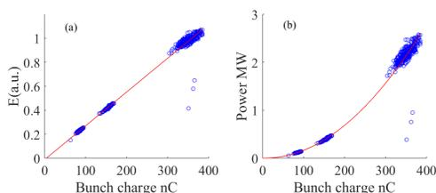
Figure 6: The measured rf signal (a) and the derived power (b) at the backward coupler as a function of the transmitted charge when driven by 8-bunch trains. The red line in (a) represents the linear fitting of the experiment data. The red line in (b) uses the same fitting results in (a) to calculate the power.
