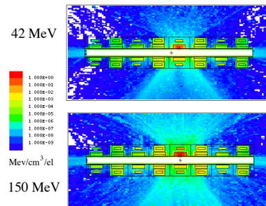
Figure 6: Radiation dose pattern in the yz-plane produced by 42 and 150 MeV electrons hitting the vacuum at the center of magnet QF3 at an angle of 10° in Figure 3
