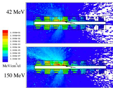
Figure 4: Radiation dose pattern in the yz-plane produced by 42 and 150 MeV electrons hitting the vacuum at the center of magnet BD2 at an angle of 10° in Figure 3.
