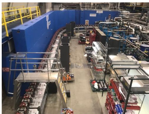
Figure 2: Photo of the straight section of the permanent magnet FFA return loop.
