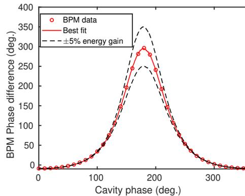
Figure 4: Change of the arrival phase time of the beam (shown as a phase change with respect to the RF clock) as a function of main linac cavity 6 phase set-point at a constant cavity gradient. Measured points are shown compared to the best fit model, and models that have  $\pm 5\%$  energy gain.
