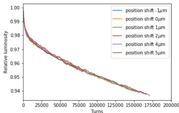
Figure 4: Luminosity degradation of various closed orbit via external control.
