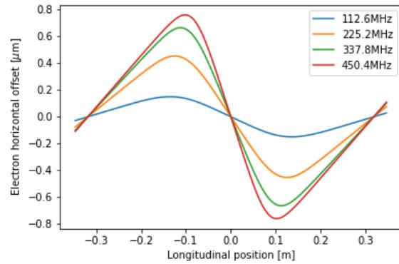
Figure 1: Trajectories of electron reference particle with different ion crab cavity frequency. Top: fresh electron with on-axis orbit before beam-beam interaction. Bottom: electron reference particle's closed orbit.
