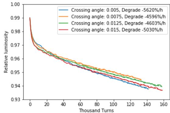
Figure 2: Luminosity degradation with different crossing angle.
