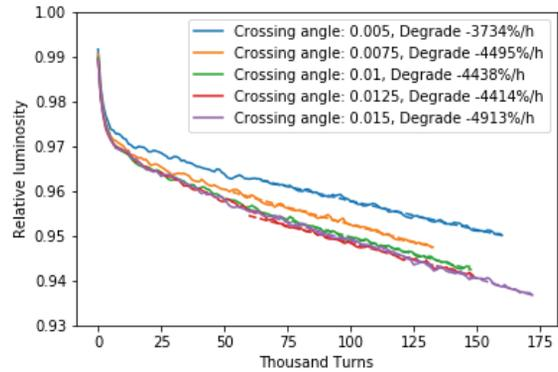
Figure 1: Luminosity degradation with different crossing angle.
