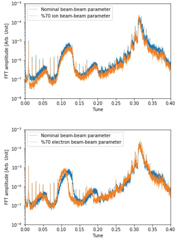
Figure 4: Frequency spectrum of the ion beam centroid with different Beam-Beam parameter of the ion beam (top figure) and of the electron beam (bottom figure).
