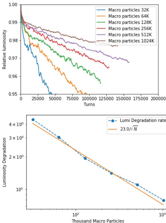
Figure 5: Scaling of luminosity degradation with the number of macro-particle used in simulation with nominal parameter, which leads to synchro-beta resonance.
