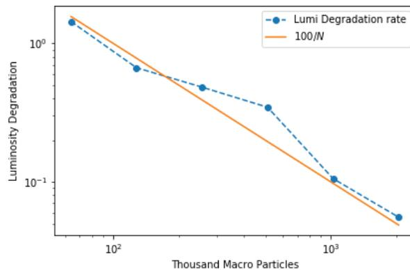
Figure 6: Scaling of luminosity degradation with the number of macro-particle used in simulation with ion synchrotron tune reduced by 10 times which significantly reduce the synchro-beta resonance.
