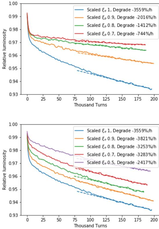
Figure 3: Luminosity degradation with different Beam-Beam parameter of the ion beam (top figure) and of the electron beam (bottom figure).
