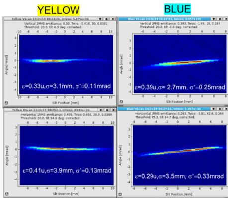
Figure 5: Transverse phase space measurements (geometrical emittance) in the two cooling sections.
