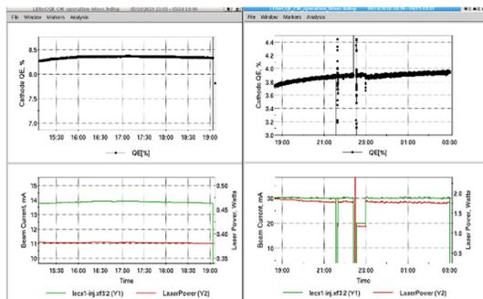
Figure 6: High current 9MHz CW operation with laser beam intensity feedback on. 1) 2018 run of 30 mA in injection line 2) 2019 run of 14 mA to the final high-power beam dump. At the bottom plot: laser average power delivered to the cathode (red) and beam current measured by DCCT (green), at the top cathode QE in % (black).
