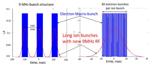
Figure 2: Thirty electron bunches (blue) spaced by 1.4 ns placed on a single ion bunch (red).
