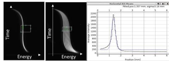
Figure 4: Longitudinal phase space measurements at RF diagnostic YAG profile monitor for a bunch charge of 75 pC, time is in vertical, energy is in horizontal axis: 1) single macro-bunch, 2) six macro-bunches train with good compensation of beam-loading effect by the 9MHz cavity, 3) horizontal profile of the center part of the single macro-bunch.
