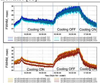
Figure 7: Bunch length reduction in both RHIC rings as a result of longitudinal electron cooling.
