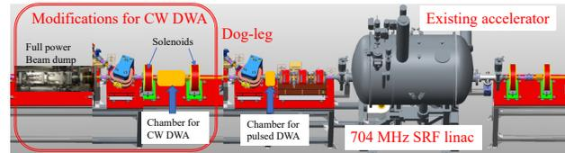
Figure 6: The end of the CeC accelerator with the quadrupole triplet and proposed modification to the system: a small chamber for initial pulsed DWA experiment and extension of the beamline for the CW DWA experiment terminated by the full power e-beam dump.
