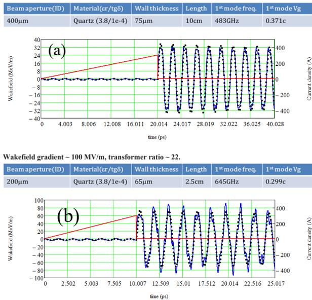
Figure 4: DWA parameters for case 1 (a) and 2 (b). Red line is the shape of the e-bunch, black dots – the wakefield of the dominant mode, blue continues line – combined wakefield of 4 dominant modes.
