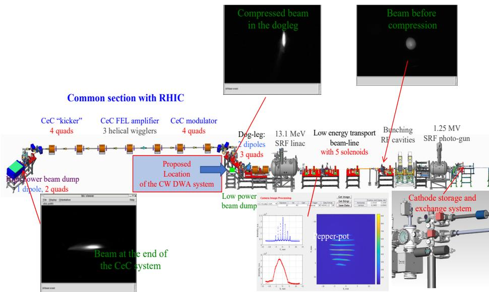
Figure 1: Layout of the CeC proof-of-principle systems at IP2 of RHIC.
