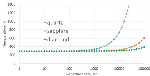
Figure 5: Steady state temperature distribution for 200 ps pulse length, 1GV/m gradient at various repetition rates.
