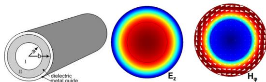
Figure 3: Partially Dielectric-Loaded Circular Waveguide: The dielectric tube has inner radius  $a$  and outer radius  $b$ .
