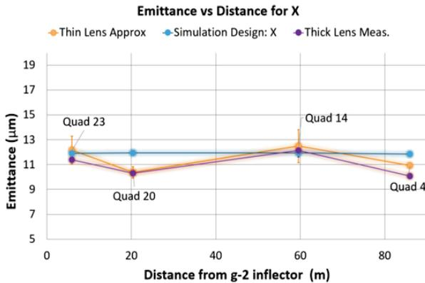
Figure 7: Emittance as a function of distance from the entrance of the storage ring of the Muon g-2 Experiment. We compared our measurements from both analysis frameworks with simulation. An extra emittance measurement was made for quad 23 using PWC25. Note that distance equal to zero points to the entrance of the storage ring.
