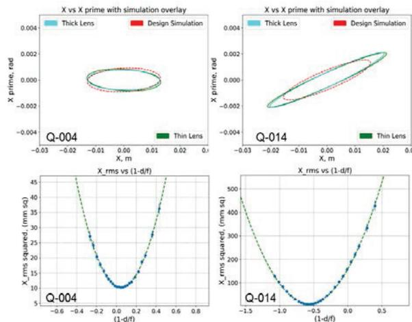
Figure 5: The phase-space and parabola plots for quadrupoles Q004 and Q014. In the phase-space plots, the dashed contours represent the phase plots from the simulation and the solid lines are from the measurement. The ellipses are generated from the Twiss parameters extracted from their respective parabola plot. Only horizontal plane is shown.
