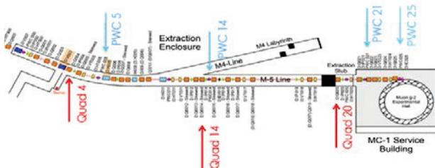
Figure 3: The M4 and M5 lines of the Fermilab Muon Campus. The quadrupoles marked are in red and the profile monitors are indicated by the blue arrows and any quadrupole in between the monitor and our quadrupole of interest is turned off. At the end of the M5 line is the g-2 storage ring in experimental hall MC-1.
