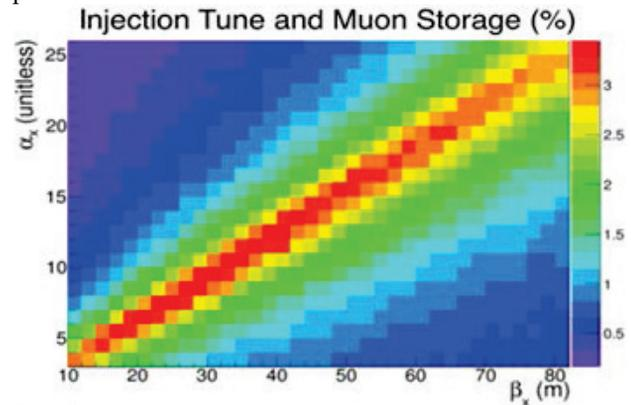
Figure 1: Example of Twiss parameters at injection and the corresponding muon storage. Injection is most sensitive to horizontal Twiss parameters since the narrowest aperture is  $\Delta x = \pm 9\text{mm}$ .
