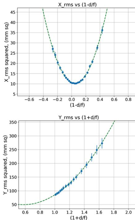
Figure 4: Thin lens parabolas for quadrupole 4 where the top plot (full parabola) goes through a waist in the X direction and the bottom plot (half parabola) does not have a waist in the Y direction.
