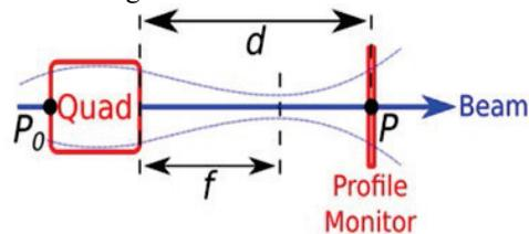
Figure 2: Diagram of the quad-scan setup. d is known as the drift distance and f is the focal length of the quadrupole. The Twiss parameters calculated from the measured beam widths describe the phase space at P<sub>0</sub>.
