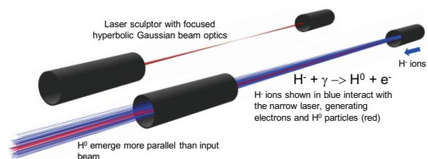
Figure 1: A *laser sculptor* modelled in BDSIM shows the simulated interaction between a narrow laser beam traversed by a larger  $H^-$  ion beam. Neutralised ions are sculpted from the core of the  $H^-$  beam producing an  $H^0$  beam with reduced emittance defined by the geometrical overlap with the laser.
