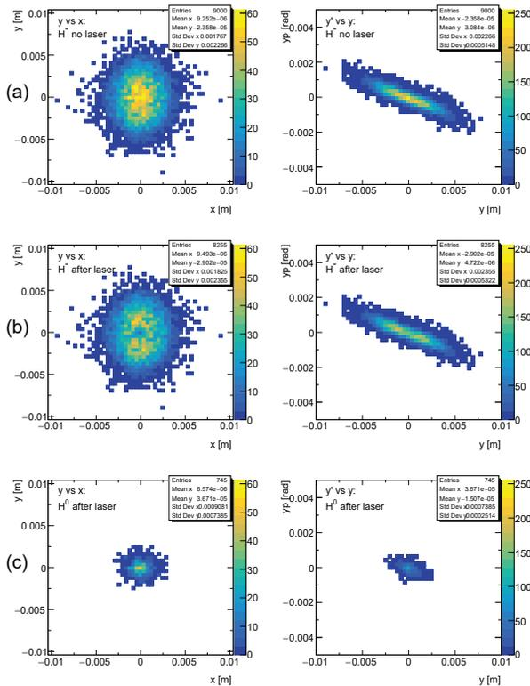
Figure 2: 160 MeV LINAC4  $H^-$  beam: (a) no laser, (b) with laser and (c) the  $H^0$  extracted by single pass laser sculpting.
