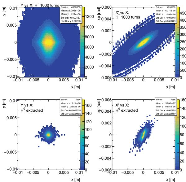
Figure 6:  $H^-$  beam for 1000 turns of the racetrack is extracted as  $H^0$  by the laser sculptor with reduced size and emittance.
