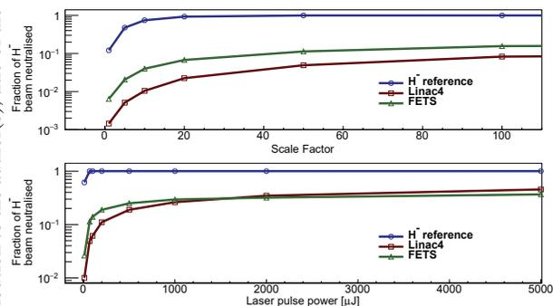
Figure 4:  $H^-$  single pass stripping efficiency through a 1 m long,  $w_0 = 0.1$  mm laser sculptor as the interaction probability scale factor and laser pulse power are varied.
