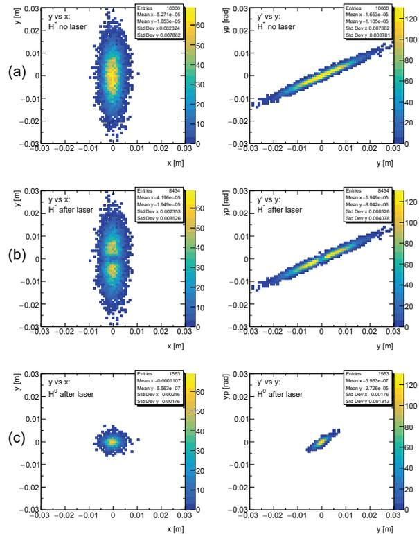
Figure 3: 3 MeV FETS  $H^-$  beam: (a) no laser, (b) with laser and (c) the  $H^0$  extracted after single pass laser sculpting.
