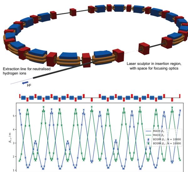
Figure 5: Racetrack storage ring with laser sculptor in red (beam pipe section invisible for visualisation) and the extraction line for neutralised hydrogen ions, emerging in blue.
