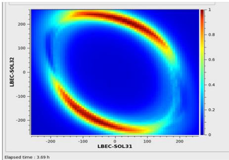
Figure 5: LEBT solenoid scan for the  $25\mu\text{A}$   $^{40}\text{Ar}^{14+}$ . The 100% transmission is reached in the dark red region.
