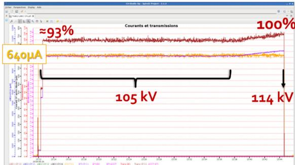
Figure 4: CW operation with  $650\mu\text{A}$   $^{18}\text{O}^{6+}$  beam. Beginning with 105 kV and finishing with 114 kV. The red line is the RFQ transmission, orange the beam current before RFQ, violet the beam current after the RFQ.
