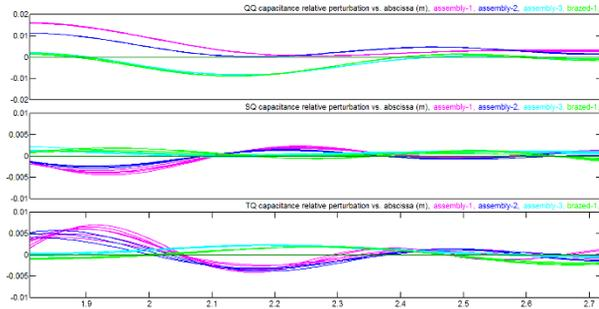
Figure 3: Comparison of beadpull measurements for Section 3 manufacturing.
