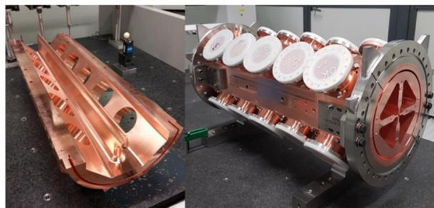
Figure 1: Major vane and finished section.
