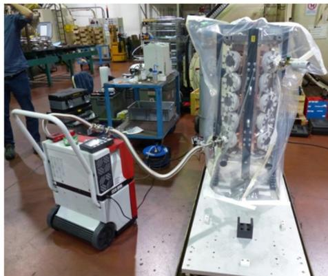
Figure 2: Leak test of section.
