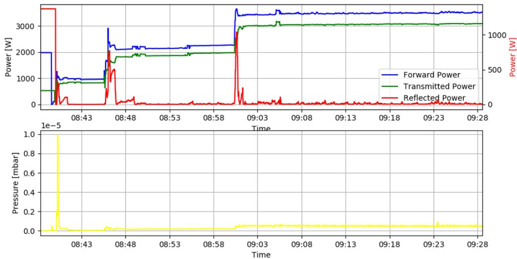
Figure 3: Measured power and pressure data for the commissioning of CH 1 up to 3 kW.
