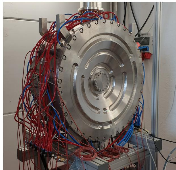
Figure 4: CH 1 in the bunker of the experimental hall of the IAP with connected vacuum and cooling water system including temperature monitoring.
