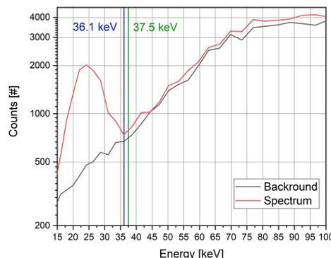
Figure 5: The measured x-ray spectrum of the RFQ for a forward power of 80 kW (red) and the background spectrum (black). Shown is the number of counts of photons as a function of their energy.
