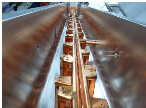
Figure 1: The electrodes inside the RFQ, as seen from the high energy end. On the right, the tuner and a pick-up loop can be seen.
