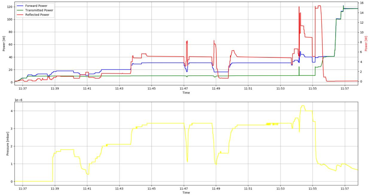
Figure 2: Measured power and pressure data showing the multipacting barrier observed at 20 W.
