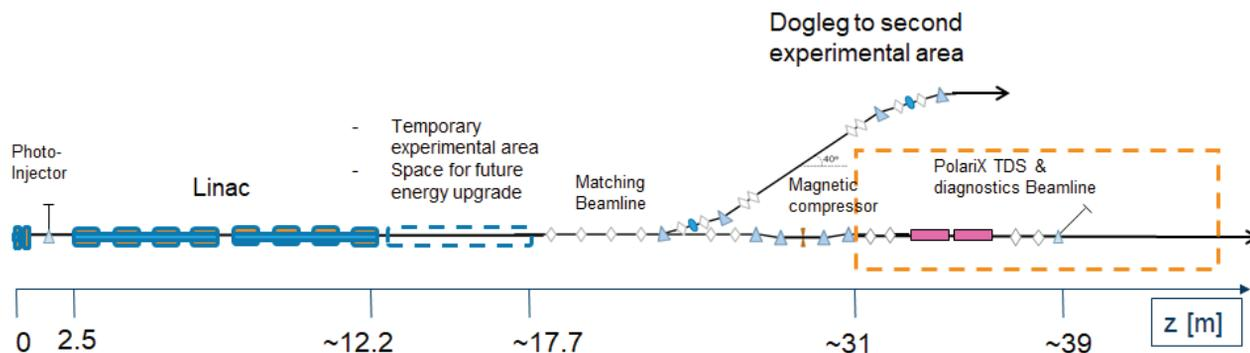
Figure 1: Layout of the ARES linac at SINBAD.
