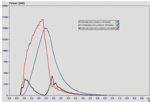
Figure 5: Forward (red), reflected (black) and RF probe pulse (blue) in the gun cavity. The RF pulse duration is 0.5  $\mu$ s. The modulator operates at a pulse width of 6  $\mu$ s and a charge voltage of 1200 V.
