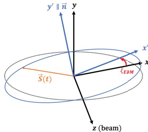
Figure 1: Due to a permanent EDM the invariant spin axis tilts in horizontal direction by the angle  $\xi_{EDM}$ .
