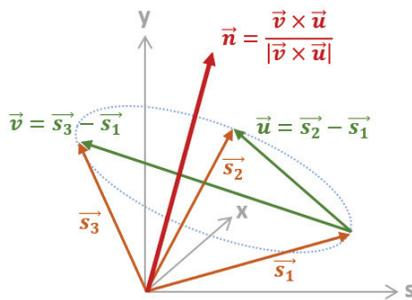
Figure 2: Method for calculating the invariant spin axis from three chosen spin vectors.
