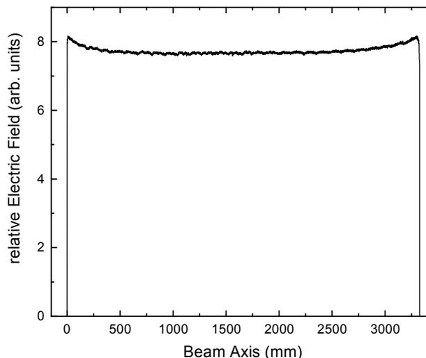
Figure 4: Flatness after tuning. The relative on-axis flatness is 1%.
