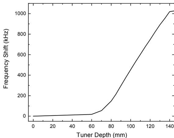
Figure 6: Tuning Range of the static tuners.
