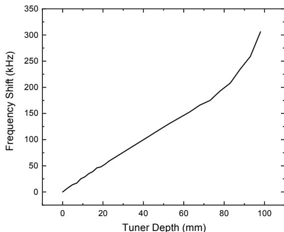
Figure 7: Tuning Range of the movable tuners.
