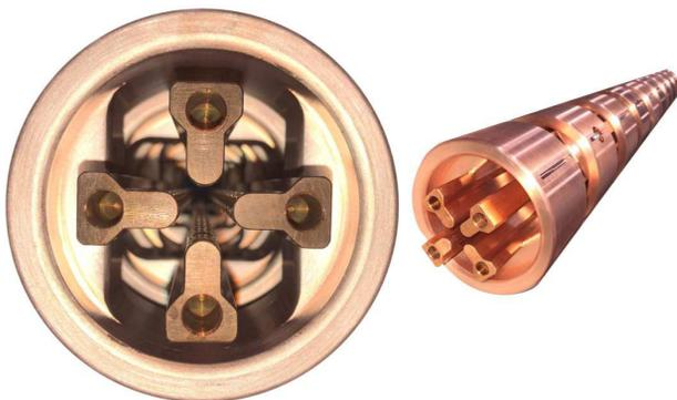
Figure 5: Electrode “basket” of the re-produced electrodes for the second tank section.
