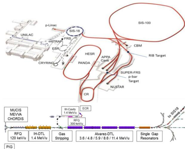
Figure 1: GSI / FAIR facility and the UNILAC injector.
