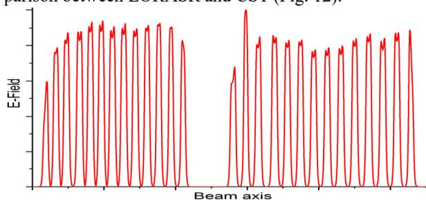
Figure 11: Simulated electrical field distribution along the beam line after changing the tuner positions.
