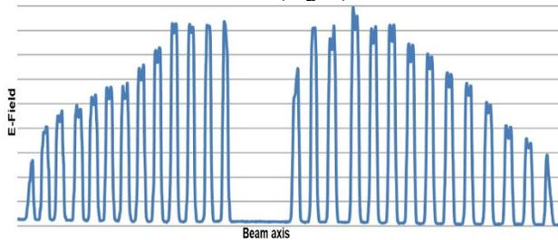
Figure 5: Measured electrical field distribution along the beam line (done in 2015 by M. Vossberg).
