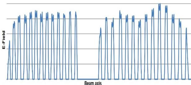
Figure 6: Best measured electrical field distribution along the beam line with tuning bodies (done in 2015 by M. Vossberg).
