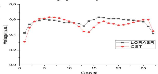
Figure 12: Voltage distribution along the beam line after changing the tuner positions (blue: LORASR and red: CST).
