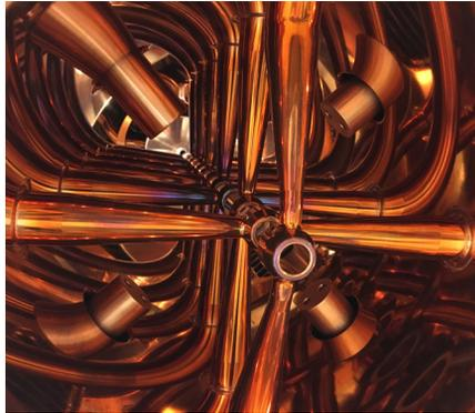
Figure 4: Copper plated inner surface of the coupled CH-prototype cavity [3].
