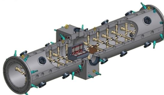
Figure 3: 3D-model of the coupled CH-prototype cavity [4].
