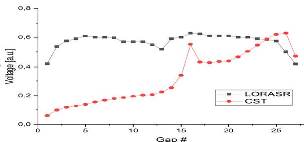
Figure 10: Voltage distribution along the beam line (blue: LORASR and red: CST).
