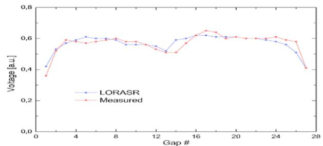
Figure 7: Voltage distribution along the beam line (blue: LORASR and red: Measurement) (done in 2015 by M. Vossberg).
