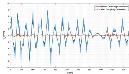
Figure 7: Vertical dispersion before and after coupling correction.
