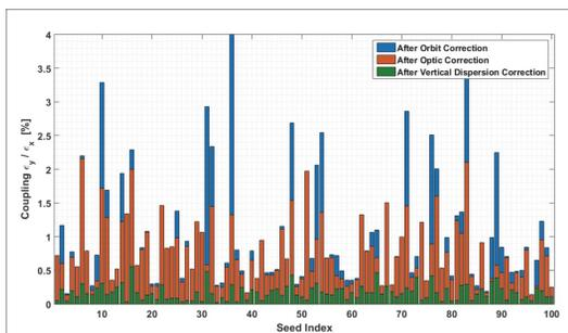
Figure 8: Coupling ratio before and after coupling correction for 100 random seeds.
