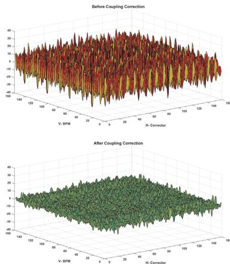
Figure 6: Off-diagonal part of response matrix before and after coupling correction.
