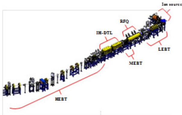
Figure 2: Layout of Linac injector.
