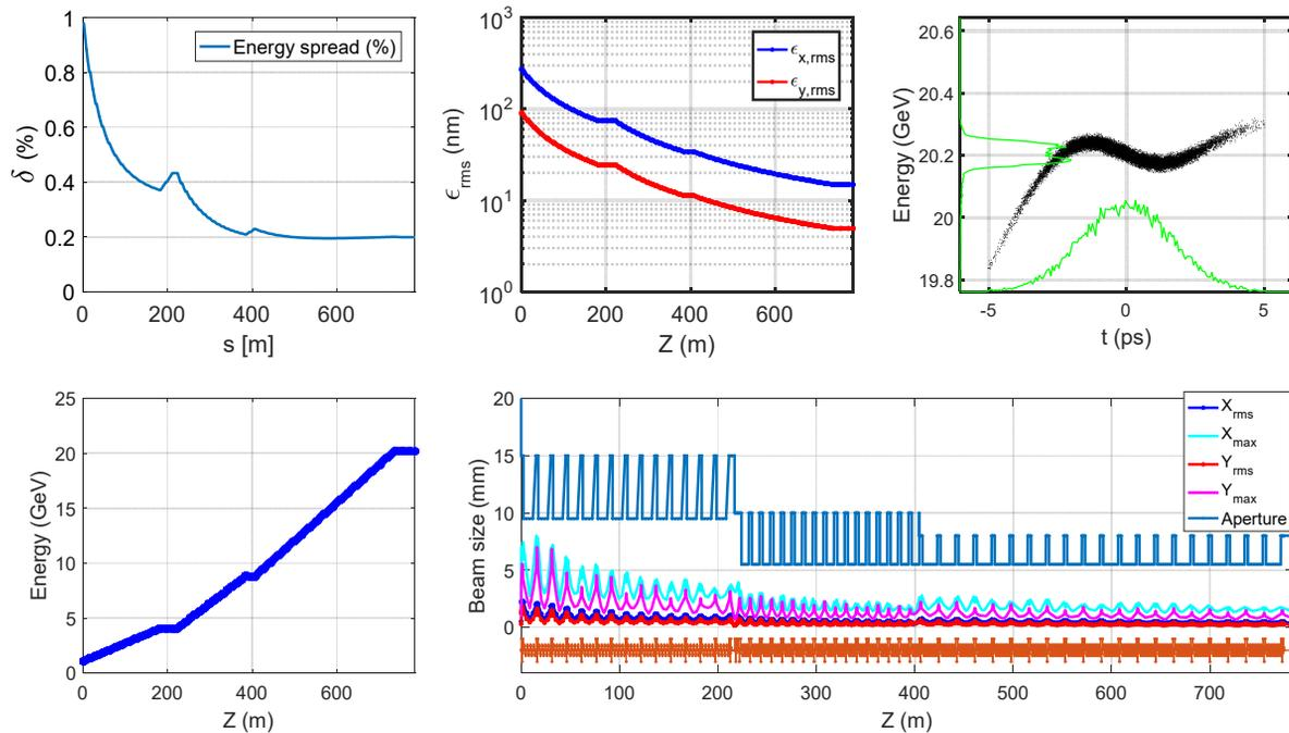
Figure 5: Beam dynamic simulation results of positron Linac: rms energy spread (top left), rms emittance (top middle), longitudinal phase space distribution (top right), energy (down left) and beam sizes (down right).
