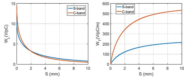
Figure 3: The short-range Wakefield of S-band and C-band accelerating structure.
