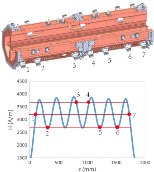
Figure 2: Positions of tuners relative to (top) the coupling windows and (bottom) the magnetic field distribution.
