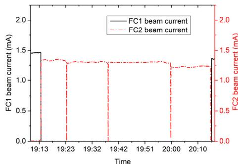
Figure 7: Change of FC1 and FC2 beam current during one hour of CW operation.
