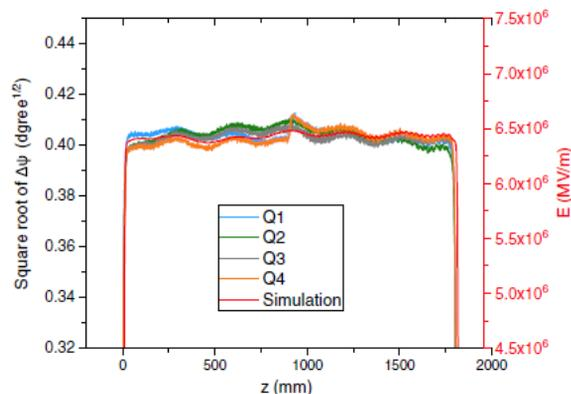
Figure 3: Measured and simulated electric field distributions after tuning.
