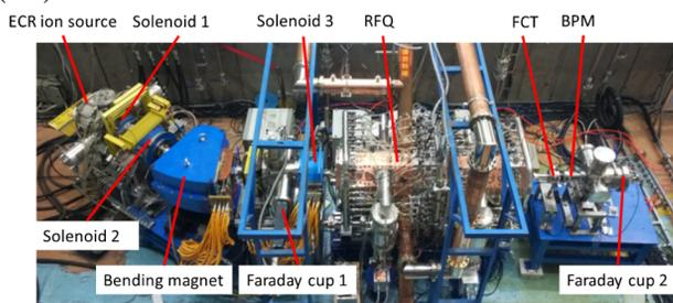
Figure 5: Overview of the RFQ test area.
