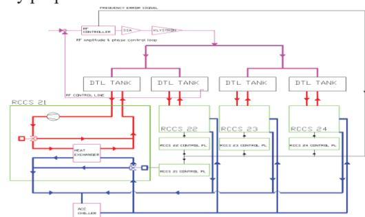
Figure 3: 20MeV radio frequency control scheme.
