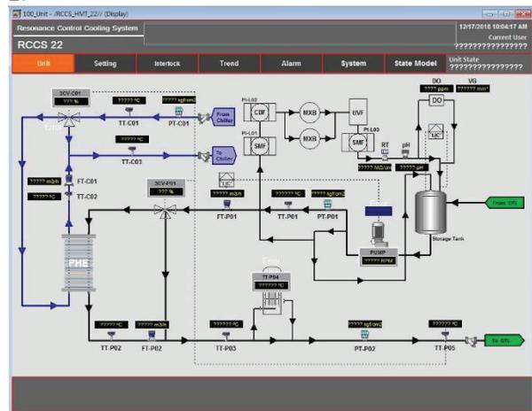
Figure 2: Piping and instrument diagram.
