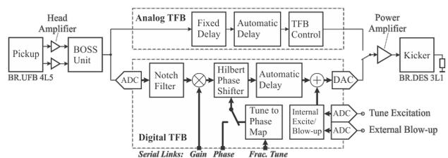
Figure 1: Simplified block diagram of the PSB TFB.
