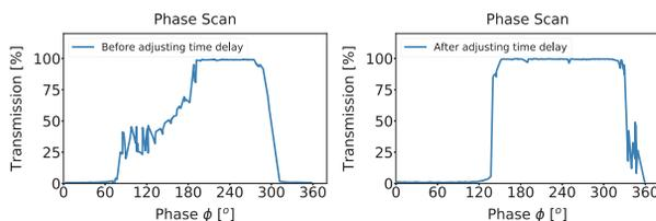
Figure 3: Example of the beam transmission recorded over the measurement plateau as a function of the phase between the TFB pickup and the TFB kicker. Left: initial setting. Right: after  $T_{FIX}$  adjustment with the VNA.
