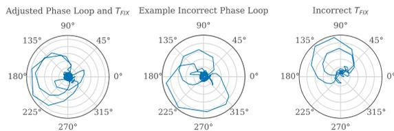
Figure 2: Example of setting up and possible misconfiguration diagnosis attainable with the VNA. Left: example of adjusted setting-up of the feedback phase and  $T_{FIX}$ . Center: example of the effect of non-adjusted feedback phase. Right: example of the effect of non-adjusted  $T_{FIX}$ .
