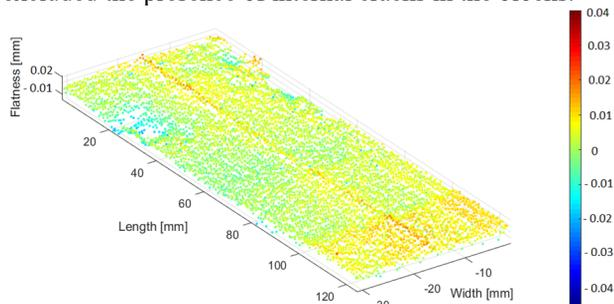
Figure 4: Flatness measurement of MoGr block #2.
