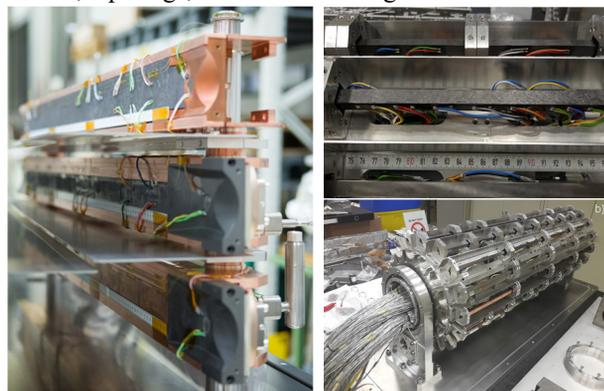
Figure 2: Configuration of Jaws, with, from top to bottom, CFC, MoGr and CuCD jaws (left) and Multimater (right).
