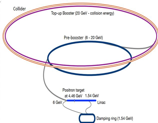
Figure 1: Layout of the FCC- $e^+e^-$  injector complex [1].
