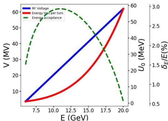
Figure 3: The energy loss per turn (red), RF voltage (blue) and energy acceptance (green) 6–20 GeV energy.
