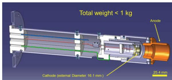
Figure 3: Longitudinal section of the optimized electron gun.
