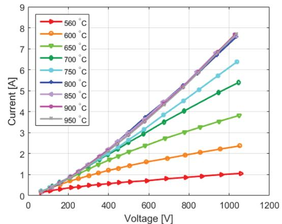
Figure 4: Current-voltage plot as a function of the different temperatures of phase 4 cathode.
