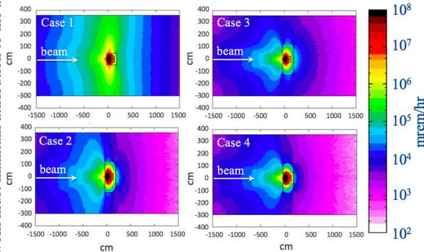
Figure 3: FLUKA results comparison between the ambient dose equivalent rates due to prompt radiation at 2 mA, 185 MeV and *Scenario A* for the four shielding cases.
