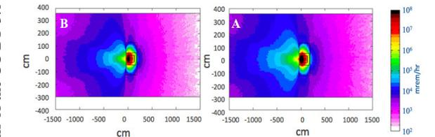
Figure 5: FLUKA Case 4 results comparison between beam pulsed *Scenario A* (right) and *Scenario B* (left) at 185 MeV. Restriction to access still applied, based on *Scenario B* results. However, access restricted to authorized personnel can be allowed during beam-on operation if a rigid barrier with locked gates is installed at approximately 15 m downstream the beam absorber.
