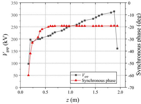
Figure 6: Gap voltage and synchronous phase of IH-EMQ.
