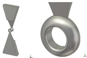
Figure 2: Model of the single cell and drift tube of IH-EMQ.
