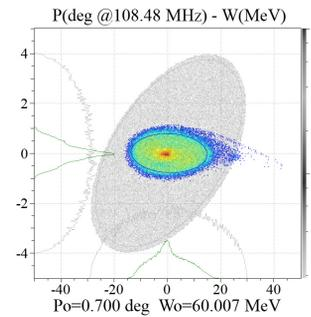
Figure 8: Longitudinal ellipse acceptance (shadow) of 60 MeV  $\text{Au}^{30+}$  and emittance output from the RFQ (color).
