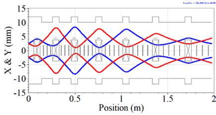
Figure 5: 2.45 times RMS beam envelope inside the IH-EMQ (blue: x-direction; red: y-direction).
