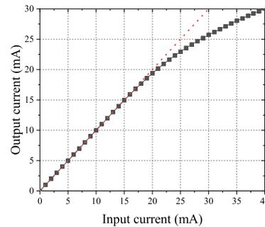
Figure 9: Current transmission for IH-EMQ.
