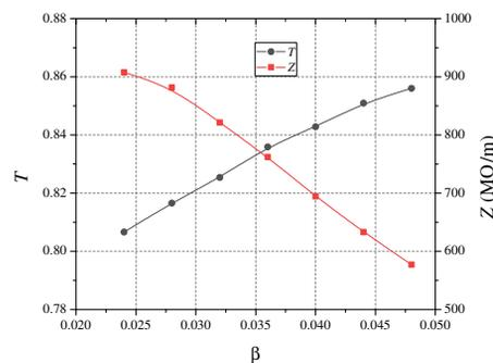
Figure 3: RF results of a single cell with different particle velocities.
