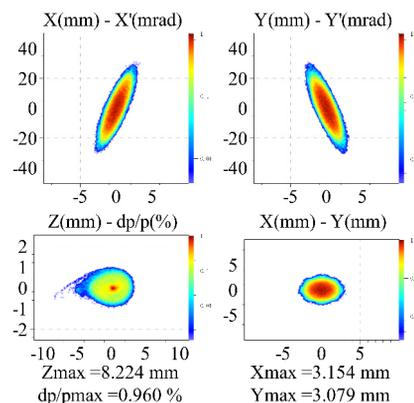
Figure 4: Phase spaces at the exit of the RFQ ( $\text{Au}^{30+}$ ).
