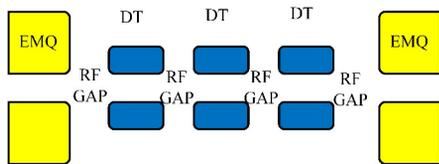
Figure 1: Sketch diagram of the typical IH-EMQ lattice.
