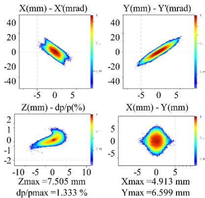
Figure 7: Phase spaces at the exit of the IH-EMQ ( $\text{Au}^{30+}$ ).
