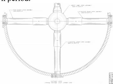
Figure 2: BNL DTL cavity with stems.
