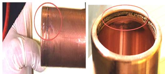
Figure 3: Damaged silver-plated beryllium copper RF spring ring in the collar.
