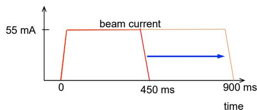
Figure 1: Doubling the average beam current by increasing the beam pulse length.
