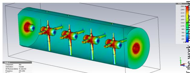
Figure 4: CST simulation of four Drift tube cavity. The RF current at spring ring are  $\sim 4000$  A/m, about 50 W per collar.
