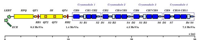
Figure 6: Layout of the HELIAC accelerator.
