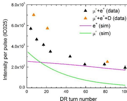
Figure 4: Total beam intensity just upstream of the entrance to the g-2 storage ring. After the fourth turn the beam in the DR contains a mixture of muons, positrons and deuterons. The green and magenta solid curves, illustrate the expected rates of muons and positrons rates, respectively.
