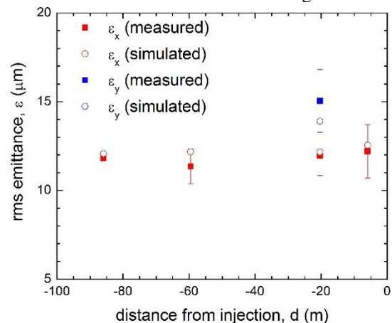
Figure 6: Emittance along the final stretch of the M5 line. Note that  $d=0$  denotes the entrance of the storage ring.
