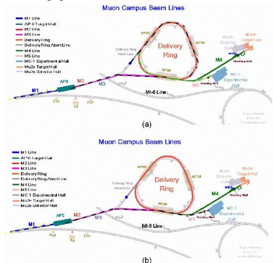
Figure 1: Muon Campus sketch: (a) During operation, and (b) initial commissioning plan. In that case, revolutions of the beam around the DR will be omitted.
