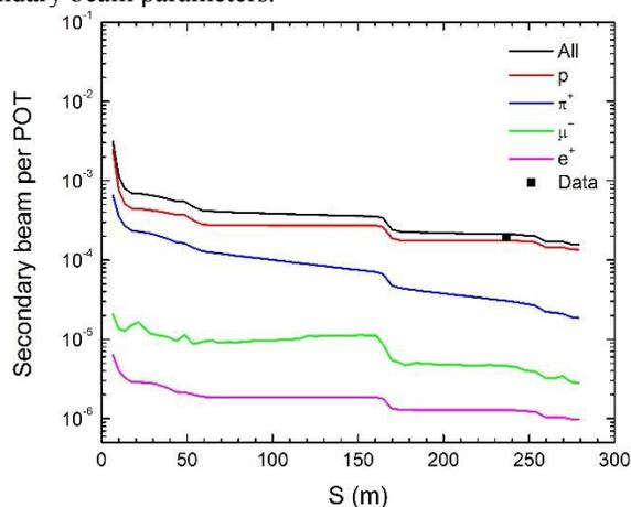
Figure 2: Simulated performance of the transmission of secondary particles. Plots for different acceptances are shown.
