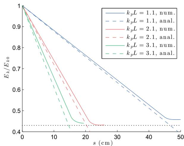
Figure 4: The beam kinetic energy  $E_k/E_{k0}$  along  $s$  for  $k_p L = 1.1$  in blue, for  $k_p L = 2.1$  in red, and for  $k_p L = 3.1$  in green. The solid and dashed lines represent respectively the numerical and analytical results.
