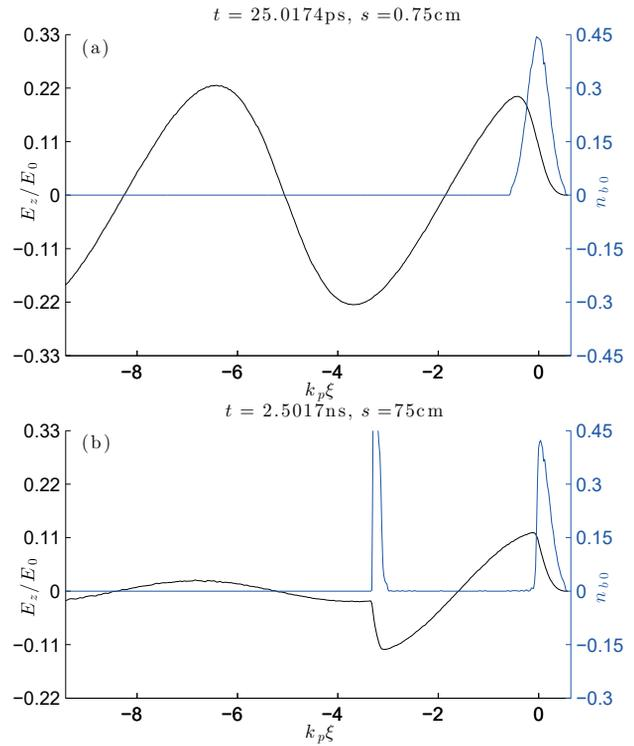
Figure 1: The beam density profile  $n_{b0}$  and the wakefield  $E_z/E_0$  at the initial, panel (a), and at the final, panel (b), of the simulation. Results are for  $k_p L = 1.1$ .
