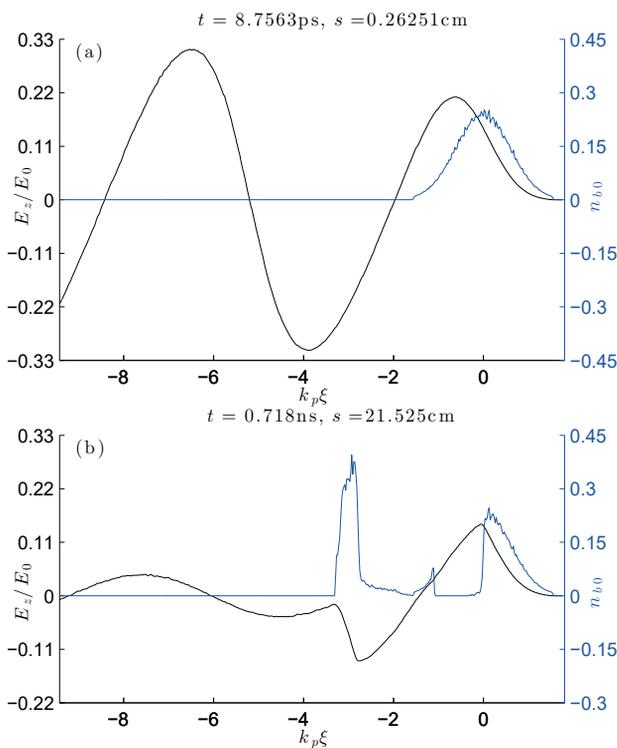
Figure 3: The beam density profile  $n_{b0}$  and the wakefield  $E_z/E_0$  at the initial, panel (a), and at the final, panel (b), of the simulation. Results are for  $k_p L = 3.1$ .
