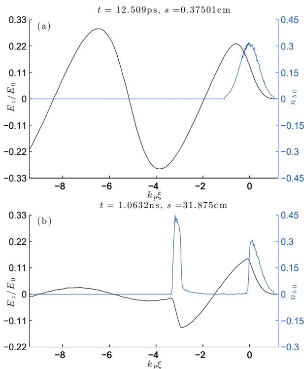
Figure 2: The beam density profile  $n_{b0}$  and the wakefield  $E_z/E_0$  at the initial, panel (a), and at the final, panel (b), of the simulation. Results are for  $k_p L = 2.1$ .
