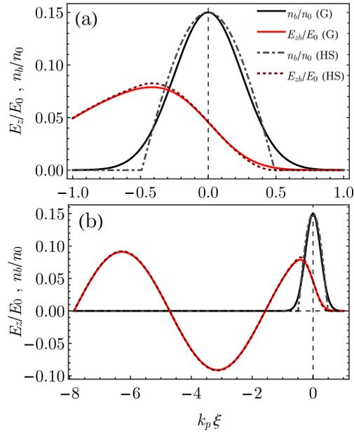
Figure 1: Gaussian and matched half-sine beam density profiles, with their respective wakefields showing good agreement. Panel (a) shows the region inside the beam, and panel (b) shows the sinusoidal wake behind the beam.
