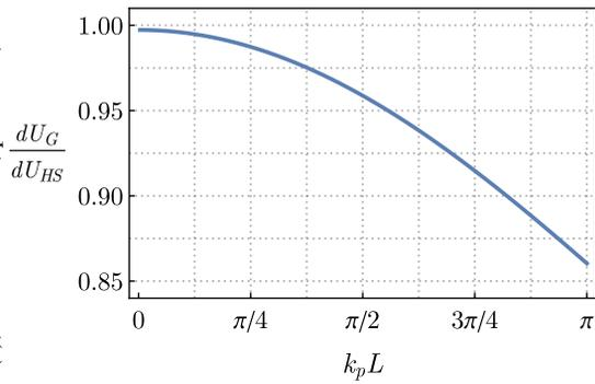
Figure 2: Ratio of total energy loss rates from the Gaussian and half-sine models, respectively. For short beams ( $k_p L \ll \pi$ ), both models are equivalent ( $dU_G/dU_{HS} \approx 1$ ). As  $k_p \rightarrow \pi$ , the ratio decreases from the unity to  $dU_G/dU_{HS} \approx 0.86$ .
