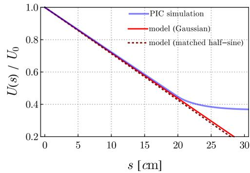
Figure 3: Total energy loss from PIC simulation (blue), Gaussian beam model (red) and half-sine beam model (darker red, dotted). Parameters are the same previously adopted.
