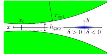
Figure 1: Geometries of a cylindrical TGU [2].
