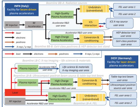
Figure 4: Simplified layout of the two EuPRAXIA construction sites in Italy (top) and Germany (bottom). Both electron beam requirements, including low energy spread and emittance, they are based on the same beamline and beam-driven and laser-beam driven cases are possible at both sites.
