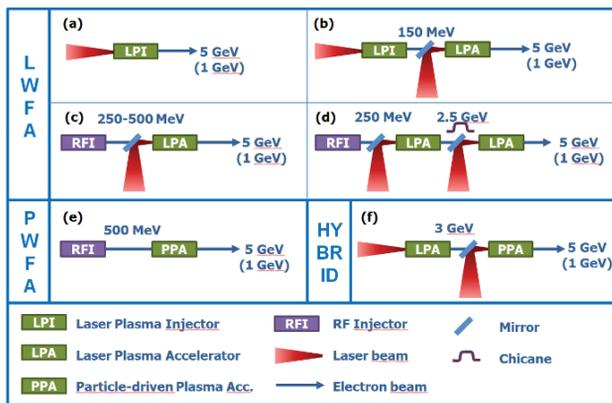
Figure 2: Overview of the injection and acceleration methods considered in EuPRAXIA. (a) LWFA with internal injection. (b/c) LWFA with external injection from a laser plasma/ or RF injector. (d) LWFA with external injection from an RF injector with two LPAs. (e) Particle-driven plasma accelerator. (f) Hybrid approach using a laser- and beam-driven plasma accelerator stage [14].
