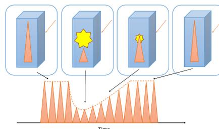
Figure 2: The typical schematic drawing of the stroboscopic method.
