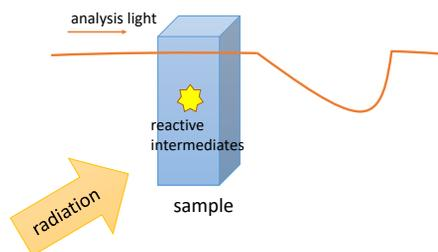
Figure 1: Scheme of the pulse radiolysis system.
