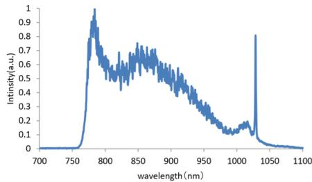
Figure 3: Spectrum band of supercontinuum light obtained from Yb doped fiber.
