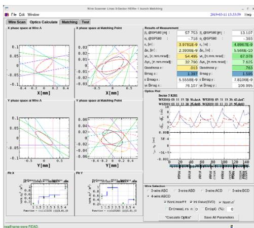
Figure 5: Emittance of electron beam at linac sector 5.
