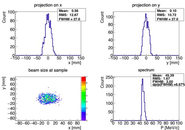
Figure 5: Decay muon beam spot and momentum distribution at sample place for 45 MeV/c.
