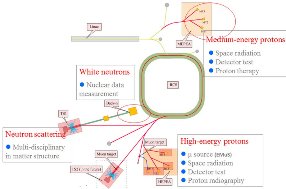
Figure 1: Layout of the CSNS and its extended beam application areas, EMuS is located in High-energy Proton Experiment Area (HEPEA).
