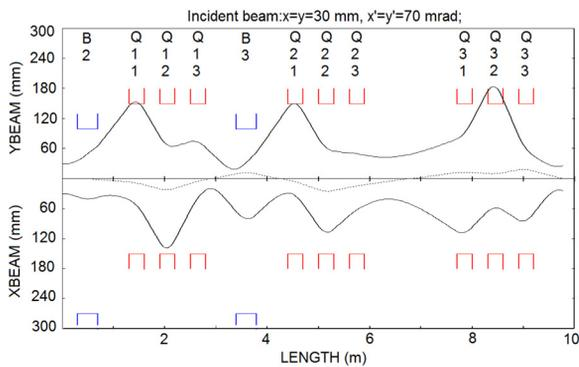
Figure 4: Beam envelopes of the beamlines after decay channel, top leading to  $\pm 60^\circ$  spectrometers, and bottom to  $0^\circ$  spectrometer.
