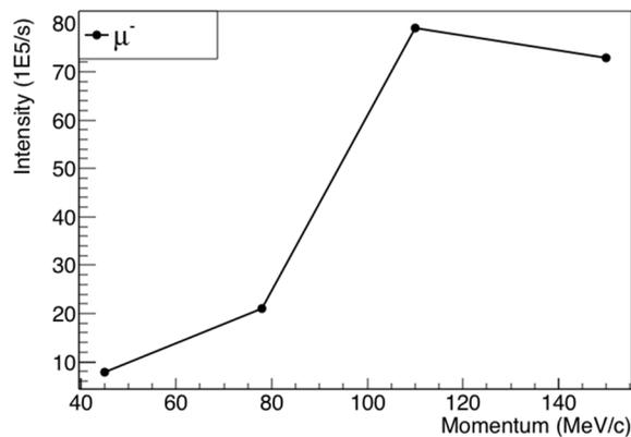
Figure 6: Negative muon intensities calculated with FWHM values on x and y around 30 mm, and momentum spread around 7%.
