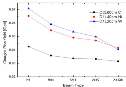
Figure 5: The production efficiency of charged pions below 200 MeV/c.
