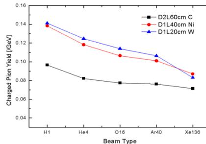
Figure 4: The production efficiency of forward charged pions within the range of 100 ~ 500 MeV/c.
