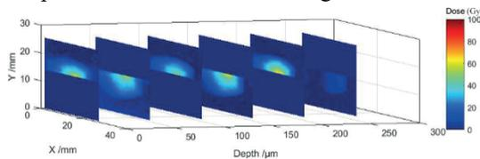
Figure 2: Dose distributions at different depths recorded on the RCF stacks.
