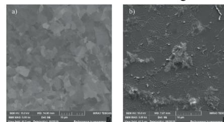
Figure 4: SEM images of the tungsten sample before (a) and after (b) laser accelerated proton irradiation.
