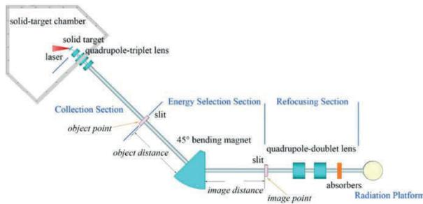
Figure 1: Layout of CLAPA Beamline.
