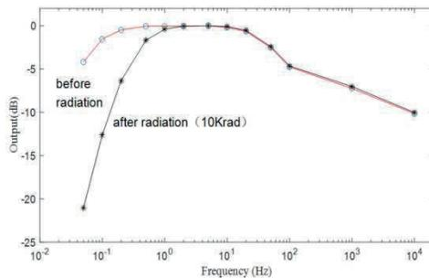
Figure 5: The response of semiconductor sensors corresponding to different frequencies.
