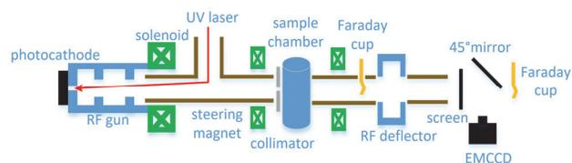
Figure 1: Schematic diagram of the MeV ultrafast electron diffraction at HUST.
