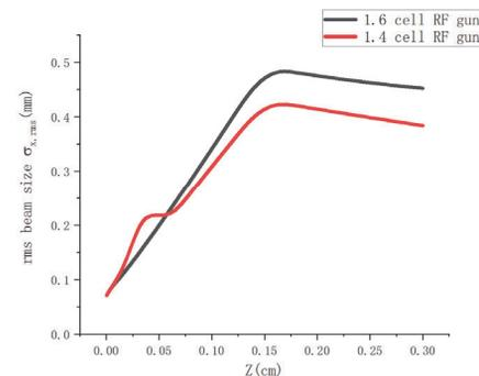
Figure 3: Simulation results of rms beam size under 1.4 cell and 1.6 cell RF gun.
