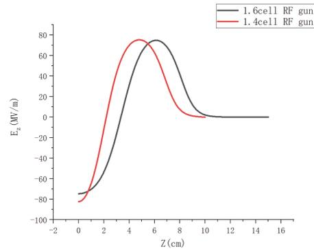
Figure 2: On-axis accelerating field of the 1.6 cell and 1.4 cell RF gun.
