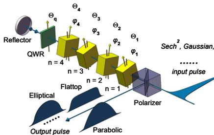
Figure 4: Physical structure of the double-pass shaper.  $\Theta_q$ , which denotes the angle between the fast or slow axis of the QWR and the polarization direction of input polarizer, equals to  $(\Theta_{N/2} + \Theta_{(N+2)/2})/2$  for a double-pass shaper, where  $N$  is the total number of BSs required by single-pass shaper. The meaning of other symbols are the same with that in Fig. 1 above.
