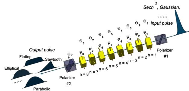
Figure 1: Physical structure of the variable shaper for arbitrary temporal shaping.  $\theta_n$  is the angle between the slow axis of the  $n$ -th BS and the polarization direction of the input polarizer #1.  $\theta_p$  is the angle between polarization directions of the output polarizer #2 and the input polarizer #1.  $\varphi_n$  is the phase delay of the  $n$ -th BS.
