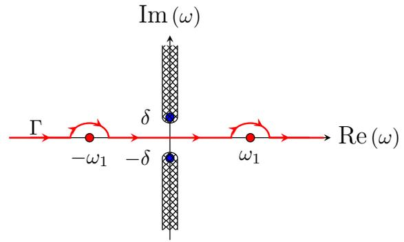
Figure 2: The location of the integration path  $\Gamma$ , the branch points  $\pm\delta$  and the poles  $\pm\omega_1$  on the complex plane  $\omega$  in the case of isotropic plasma. The hatchings denote cuts on the complex plane.
