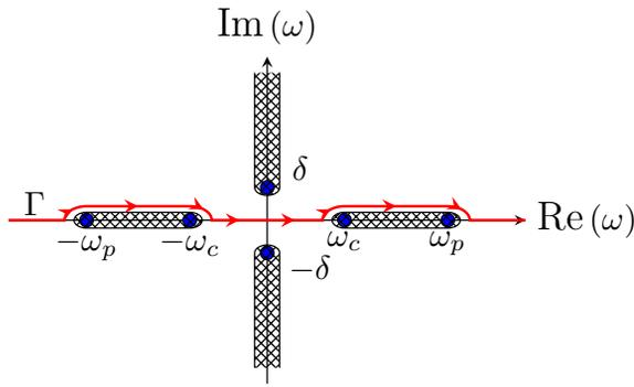
Figure 1: The location of the integration path  $\Gamma$ , the branch points  $\pm\delta, \pm\omega_{c,p}$  on the complex plane  $\omega$  in the case of magnetized plasma. The hatchings denote cuts on the complex plane.
