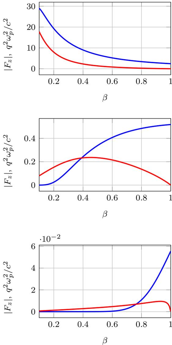
Figure 3: The dependence of decelerating force  $|F_z|$  (in units  $q^2\omega_p^2/c^2$ ) on the relative charge velocity  $\beta$  for different channel radius (top:  $a = 0.1$ , middle:  $a = 1$ , bottom:  $a = 5$  in units  $c/\omega_p$ ). Red line denotes to the case of magnetized plasma, blue line denotes the isotropic plasma.
