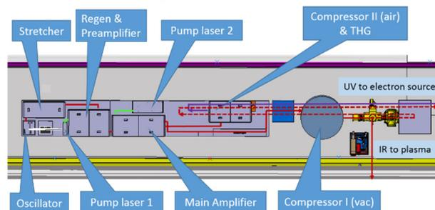
Figure 1: Layout of the AWAKE laser installation.
