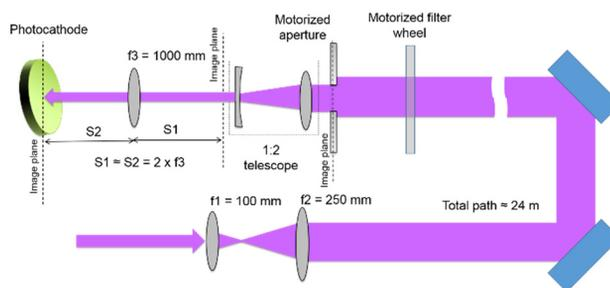
Figure 3: Simplified optical scheme of UV beam delivery to the photocathode of the AWAKE electron source.
